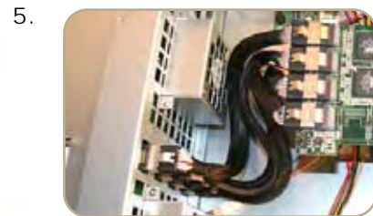
5. HDD backplane cables connected
