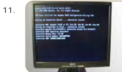
11. Your screen will show the RAID control card/ configure RAID disk and now the system is completely installed
